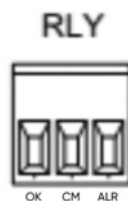
Figure 2.16 Alarm Relay Close Up
