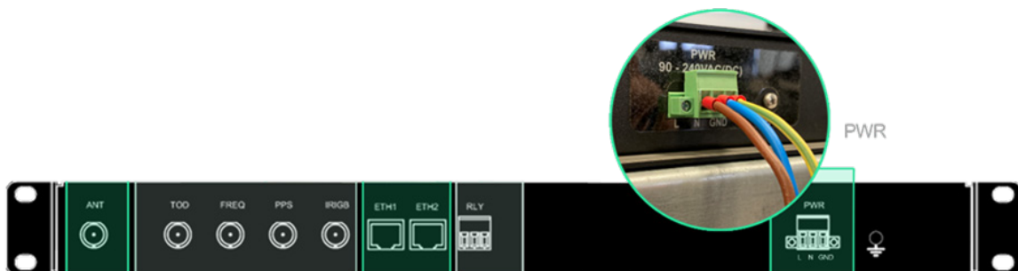
Figure 2.10 18-75 V DC Powered EKOSync 1588A Power Connection
